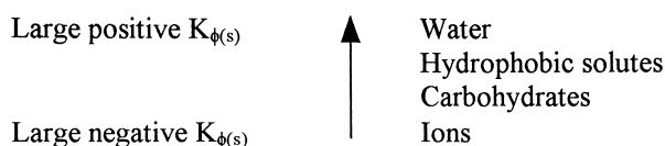
Fig. 2. Trend in isentropic apparent molar compressibility ranges of solutes in water (Source: Galema and Hoiland, 1991).
